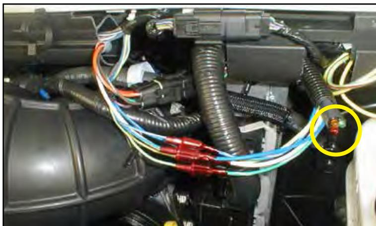
**Figure 3-2. Location of 3 Lights on Throttle Control Assembly**
